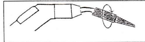
⚠ Screw the cannula by blocking it. Check. Make sure the cannula is in good shape by activating the air/water/spray functions before use in the mouth.
